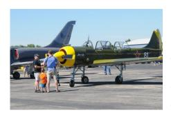
Chapter 91 member Ron Penrose owns a unique airplane: a Yak-52. Designed in Russia and manufactured in Romania, this WW-II-era military trainer served as Russia's default aerobatic competitor until very recently. The nine-cylinder Vedeneyev M14P delivers 360 horsepower, turning the prop the wrong direction.
