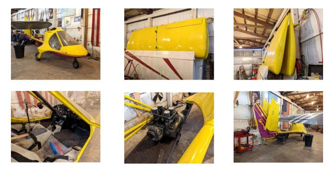
Chapter member Bruce Luedeman has an acquaintance with a rebuilding project. The plane is a two place Interplane Sky Boy, a two-seat, side-by-side, high-wing, single-engine pusher in the ultralight category. It uses a Rotax engine and is said to cruise at 128 MPH. The Skyboy was manufactured as a complete airplane by Interplane Aircraft of Zbraslavice, Czech Republic. (If you can pronounce Zbraslavice correctly, you may win a prize!)
