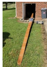
Figure 5 Minor Damage at the Tip, But a Great Spar! (Steve Schultz photo)
